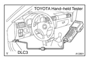
To check the DTCs, connect the OBD II scan tool or TOYOTA hand-held tester to the Data Link Connector 3 (DLC3) on the vehicle. The OBD II scan tool or TOYOTA hand-held tester also enables you to erase the DTCs and check freezed frame data and various forms of engine data (For operating instructions, see the OBD II scan tool's instruction book.).
